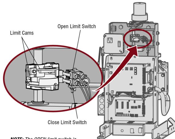
**NOTE:** The OPEN limit switch is always on the top and the CLOSE limit switch is always on the bottom.
