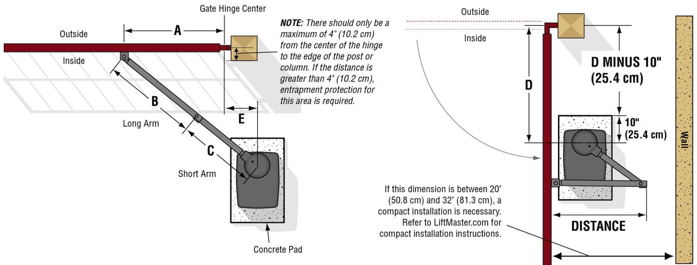
Dimension (A) thru (E) are from the center of one pivot point to the center of another pivot point.
