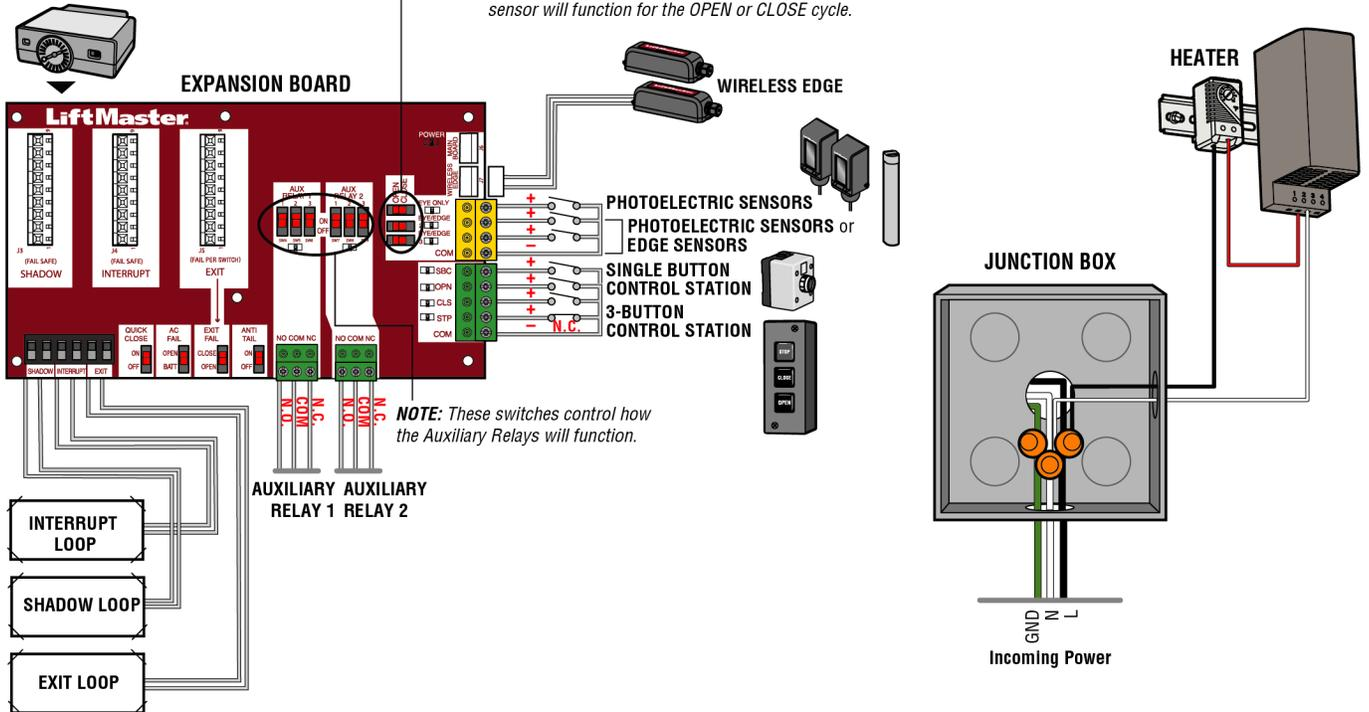
**NOTE:** These switches control how the Auxiliary Relays will function.
